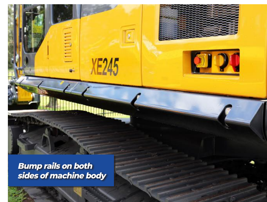
Rear of body power controls and e-stops
